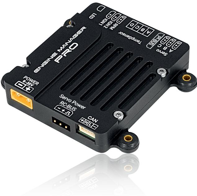
The **Engine Manager Pro** handles all tasks related to controlling and monitoring a petrol engine. Its primary functions include switching and power supply for up to two ignitions. The ignition can be supplied with **up to 35V**, while the output can be set to 6.0V, 8.0V or 12.0V. A double LC filter and overvoltage protection completely decouple the ignition supply from the rest of the on-board electronics.
